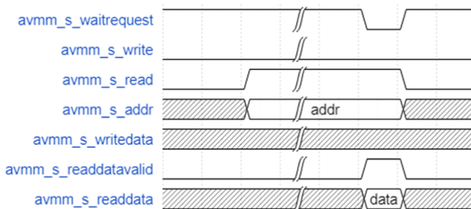
Figure 10. Avalon memory-mapped interface Master Response to a Read Request with NONBLOCKING_ACCESS_EN = 0
